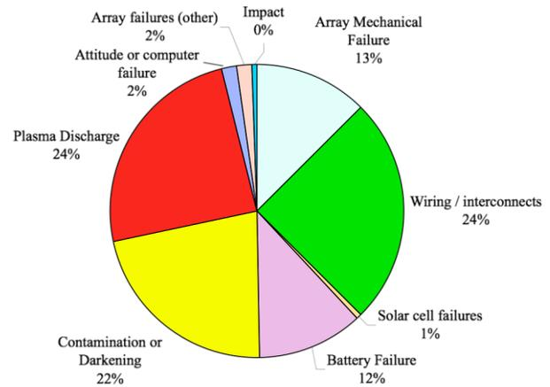
Figure 3: Cost of power-related failures, by cause.
