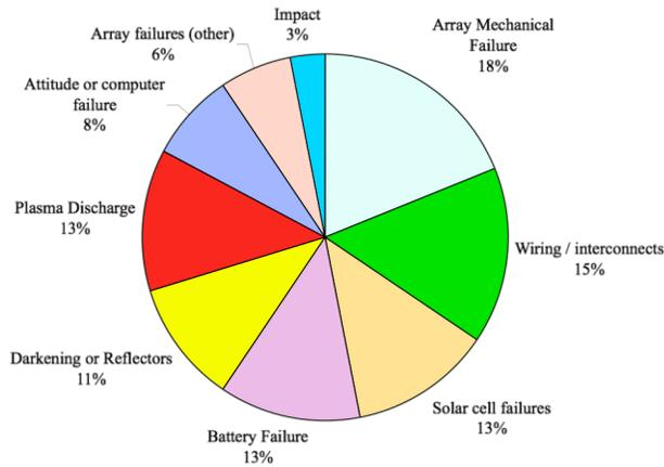
Figure 1. Number of power-related failures, by cause
