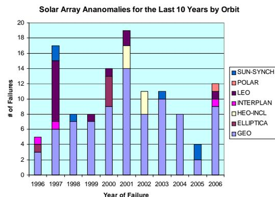
Fig. 1. Solar array anomalies by orbit
