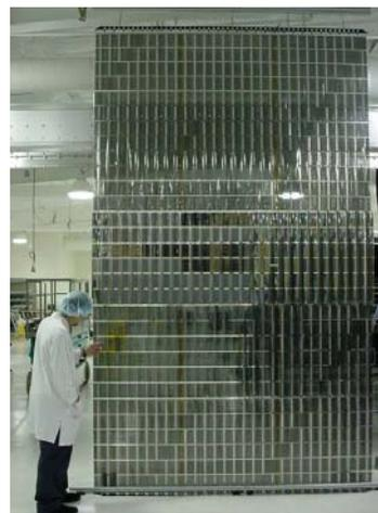
Fig. 7. A 3.75 kW Stretched lens array on a SquareRigger platform
